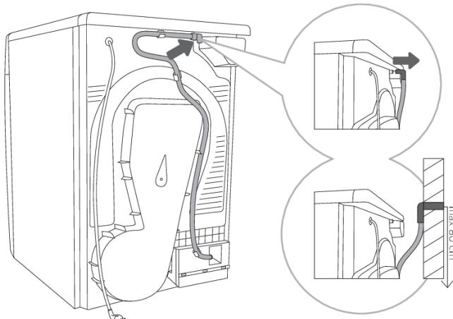
**1** Release the hose from the holder on the back wall of the dryer (left hand side, below the top cover).
