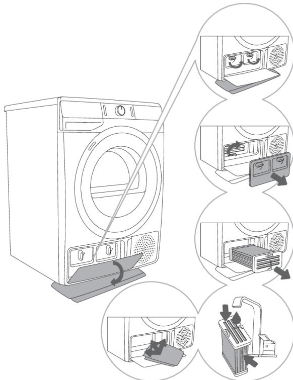
**1** Open the outer cover. Hold the levers on the inside cover and rotate them upwards.
