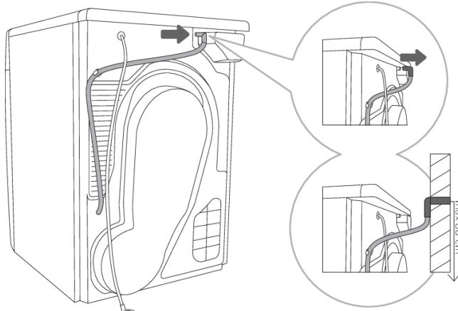
**1** Release the hose from the holder on the back wall of the dryer (left hand side, below the top cover).
