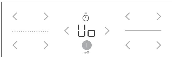
1. To activate the parameter settings menu, press and hold the key for 3 seconds while the appliance is switched off.
